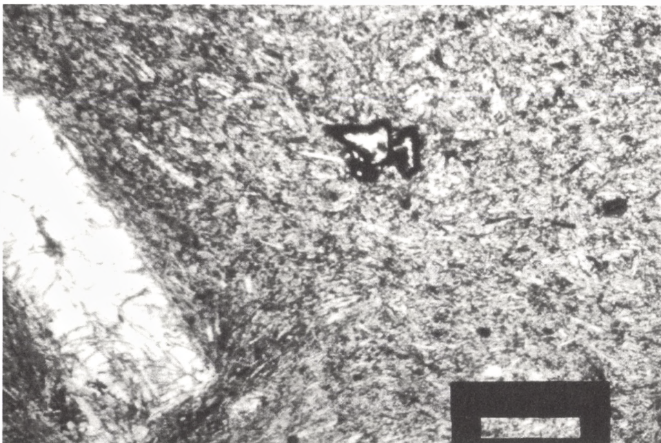
Fig. 3. Small olivine crystals with black rims and alkali feldspar phenocryst in phonolite, Puy Cordé (88-954,3), plane polarized light, scale = 0.6 mm).
